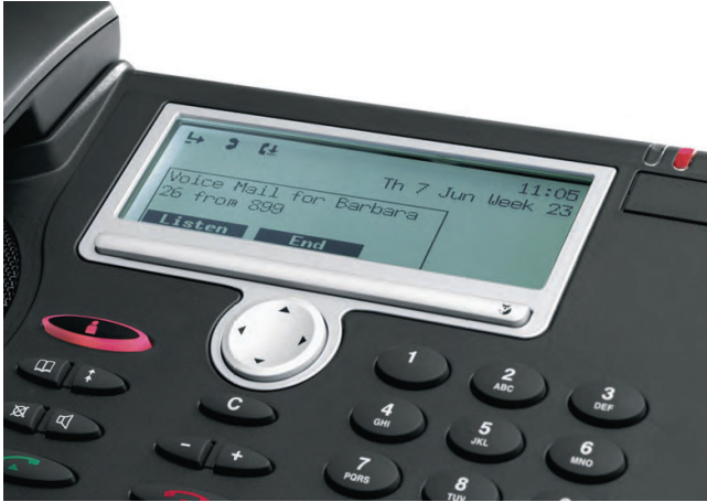
Unaccessed voice messages are displayed on screen – in this case on the Mitel 5380IP screen.
